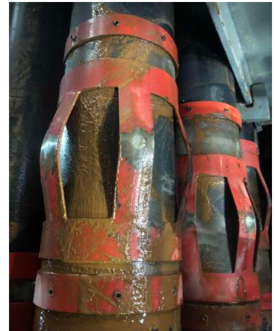
Undamaged centralizers after being POOH
