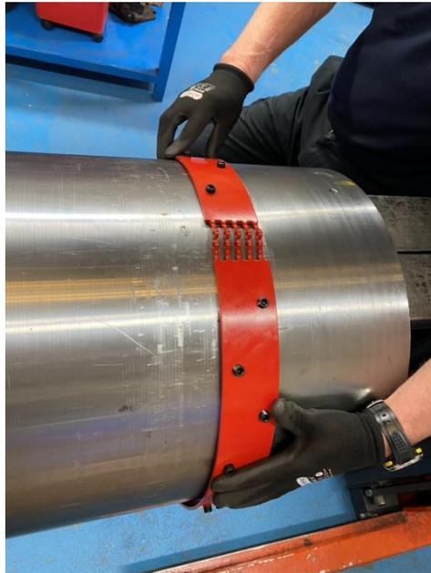
2. Manually interlock the hinge fingers, squeeze together and insert the pin into the first two fingers by hand. Ensure pin head is adjacent to centraliser.
