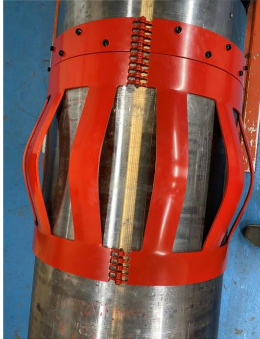
15. Remove the second collar from the pallet and wrap around the casing, approximately 2 inches above the centraliser. Ensure pin heads are adjacent to each other.
