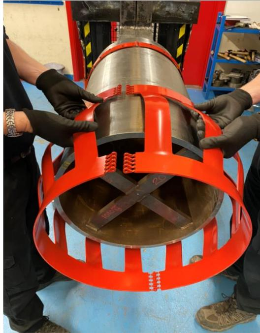
9. Interlock the hinge fingers together and using your hands, insert the pin into the first two twisted fingers. Ensure pin head is adjacent to stop collar.
