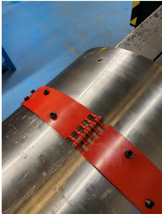
7. The installed stop collar can then be used to rest the centraliser during installation.
