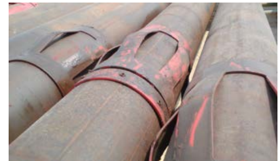
Undamaged centralizers after being POOH
