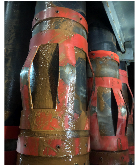
Undamaged centralizers after being POOH
