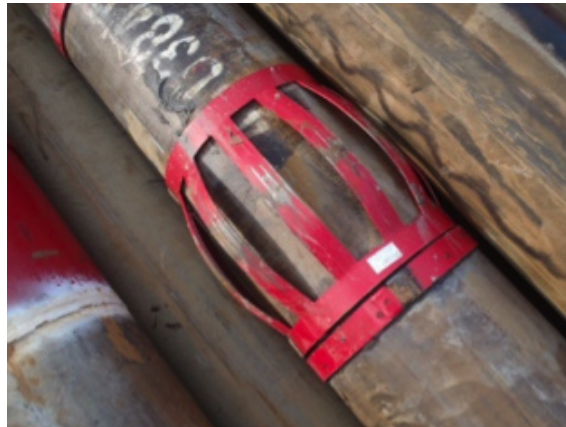
An undamaged centralizer after it had been pulled out of hole.
