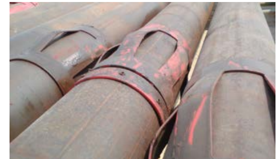
Undamaged centralizers after being POOH
