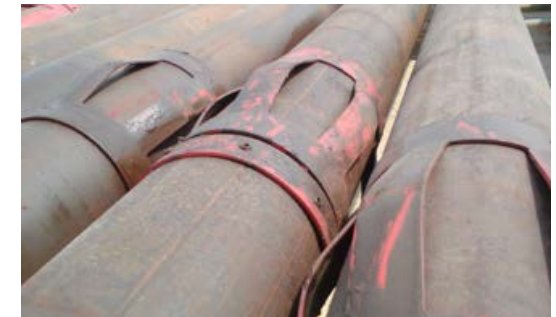
Undamaged centralizers after being POOH
