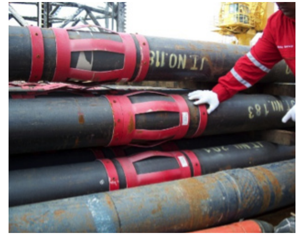
Centek centralizers on casing in yard
